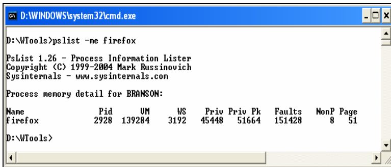
Figure 20: Using PsList to Determine How Much Virtual Memory a Process Is Using
