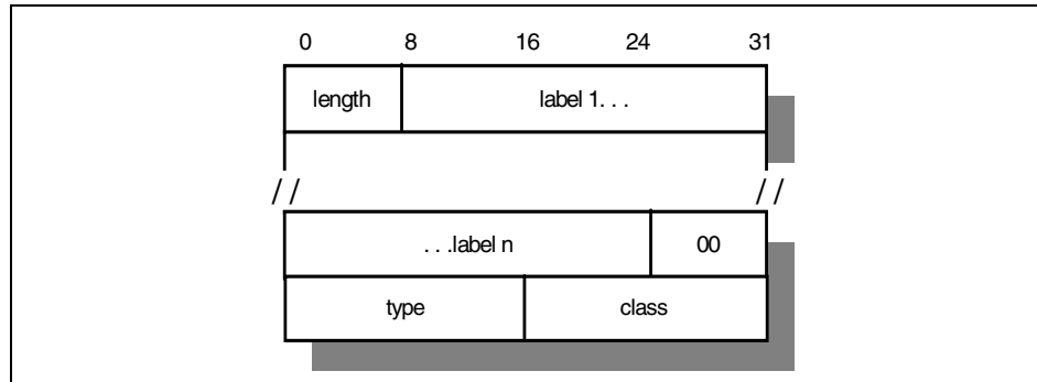
Figure 135. DNS - Question Format - all of the fields are byte-aligned. The alignment of the Type field on a 4-byte boundary is for example purposes and is not required by the format.
